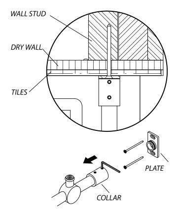
Reinstall the fixed panel assembly. Slide the collar into place.
